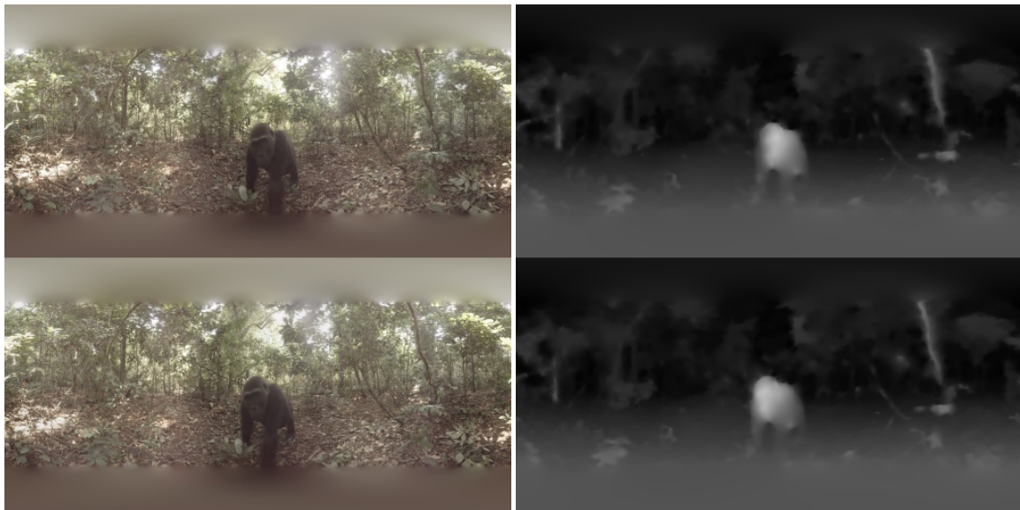
Figure 4: Example color and depth frames output from Jump Assembler.
